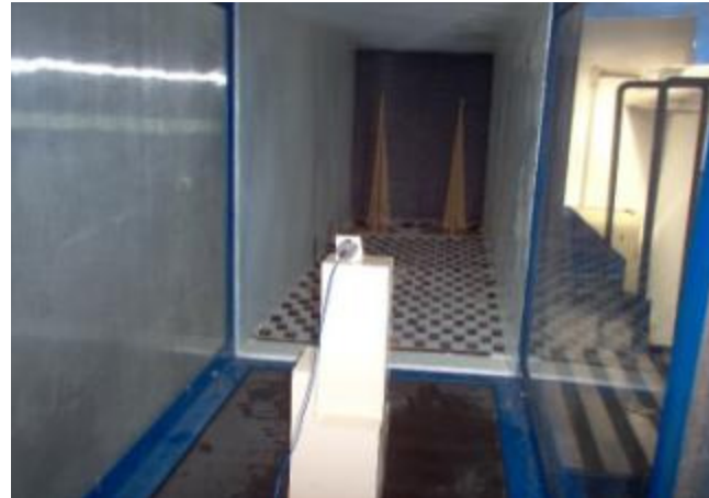
Fig. 7. Wind tunnel and instrumented scale model
