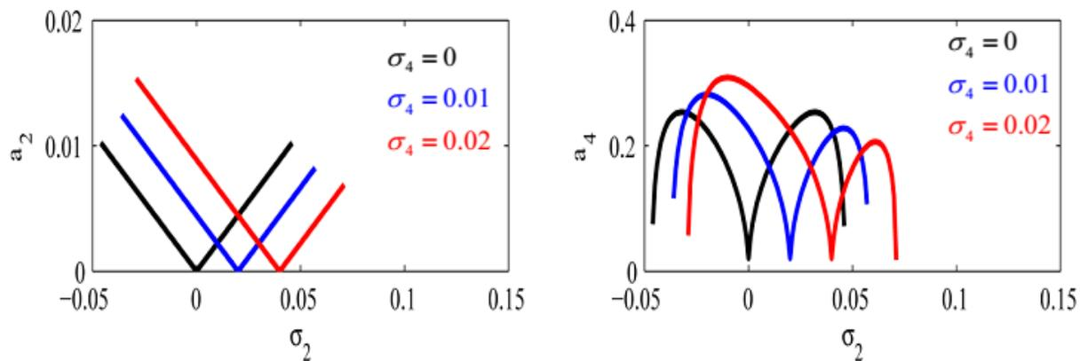
Fig.13 Influence of  $\sigma_4$  (the detuning parameter) on the fundamental system and the NSC
