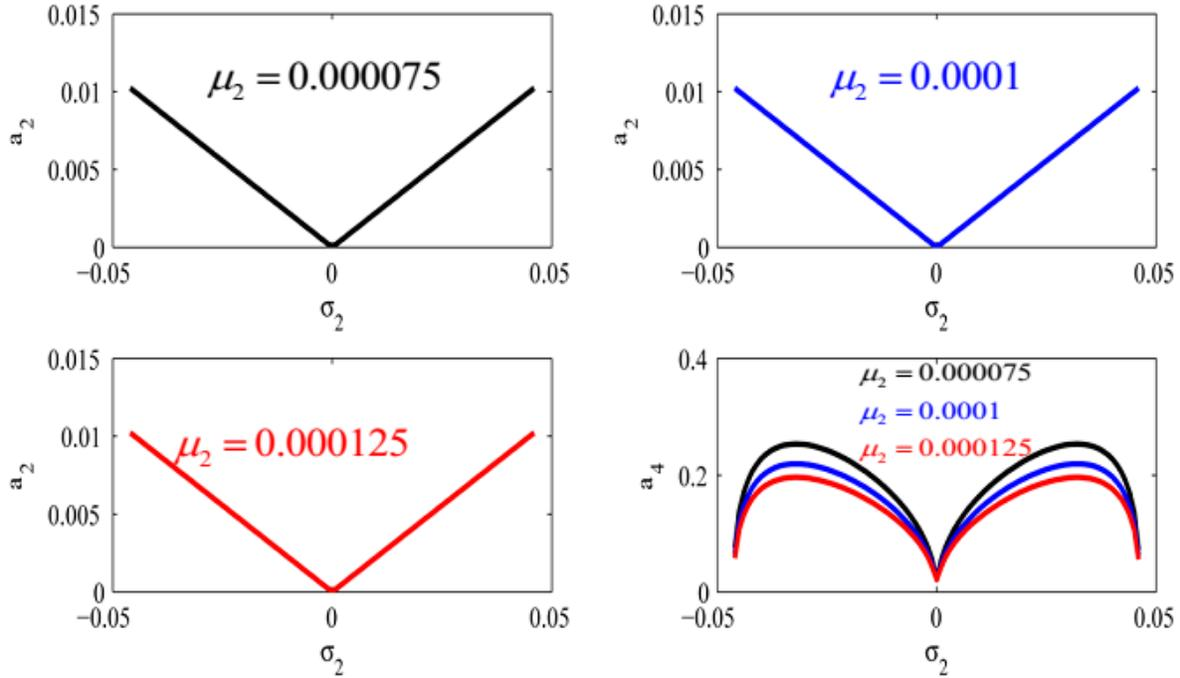
**Fig.16 Influence of  $\mu_2$  (the damping coefficient) on the fundamental system and the NSC**
