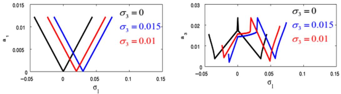
Fig.8 Influence of  $\sigma_3$  (the detuning parameter) on the fundamental system and the NSC
