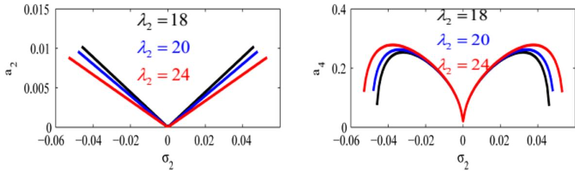
Fig.14 Influence of  $\lambda_2$  (the feedback signal gain) on the fundamental system and the NSC
