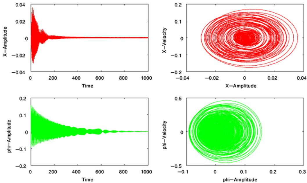
Fig.2 Response of the fundamental system with NSC controllers
