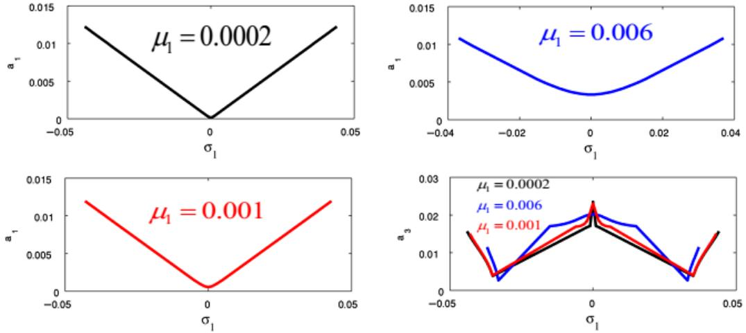
Fig.9 Influence of  $\mu_1$  (the damping coefficient) on the fundamental system and the NSC
