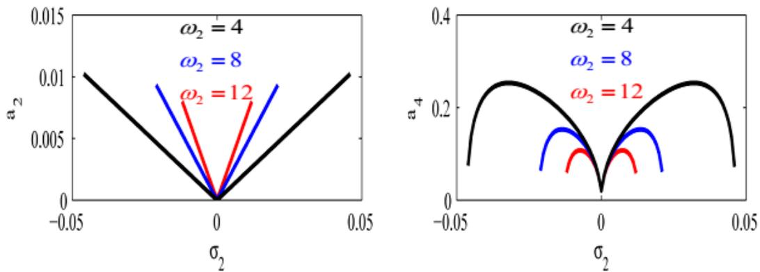
**Fig.11 Influence of  $\omega_2$  (the natural frequency) on the fundamental system and the NSC**
