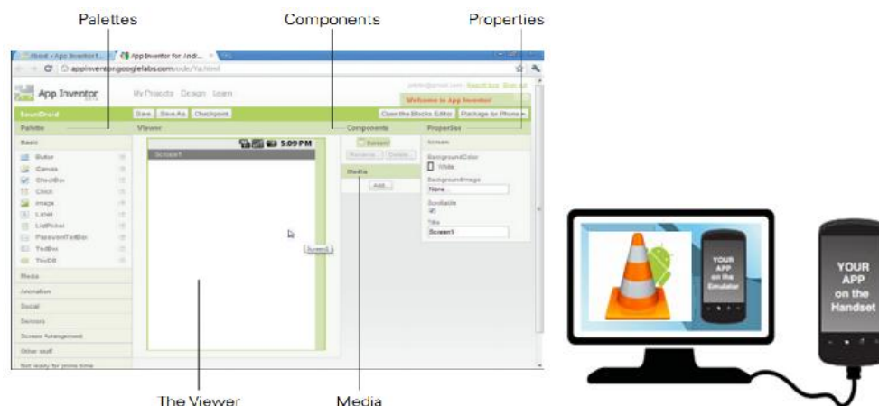
Fig. 7. App Inventor Designer (a) and the debugging perspective for an Android application using an emulator or an Android handset (b)
