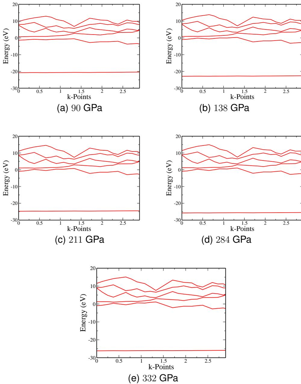
Figure 4: Change of band structure with respect to pressure at 300K
