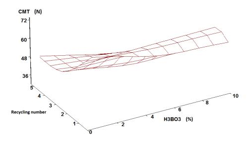
**Figure 6.** The effects of boric acid concentration and recycling phase on CMT properties of papers
