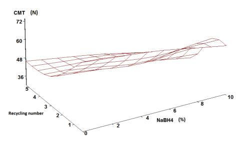
**Figure 5.** The effects of sodium borohydride concentration and recycling phase on CMT properties of papers
