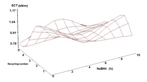
**Figure 7.** The effects of sodium borohydride concentration and recyling phase on SCT properties of papers
