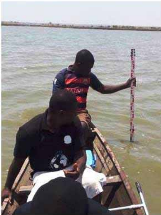
Plate 1a: Water Depth Survey
