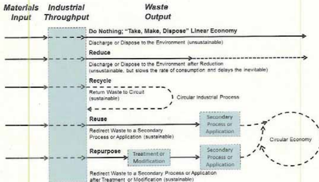
Figure 7. Relationship between materials inputs, industrial throughputs and processes, and outputs under five waste management scenarios.
