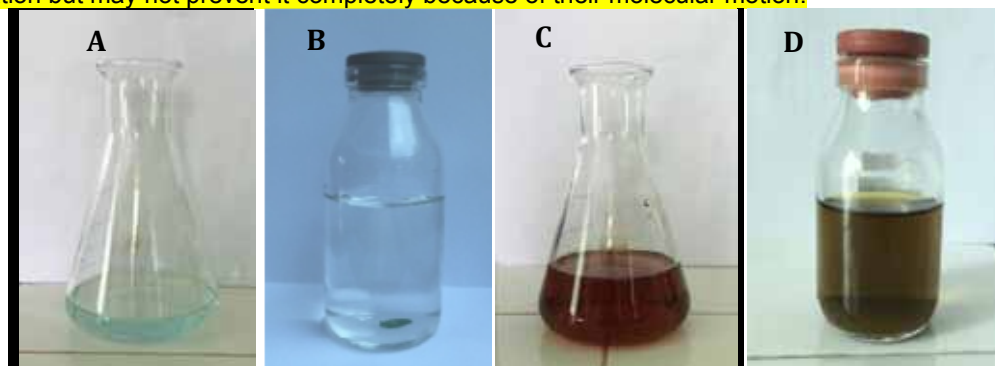
Fig. 1. Photographs of the sample: (A) CuSO 4 .5H 2 O (aq), (B) Polyvinyl alcohol (aq), (C) Mandarin peel extract and (D) Synthesized copper nanoparticles
