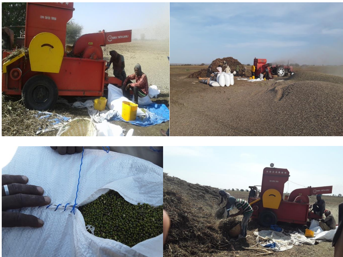
Mungbean threshing using multi crop thresher
