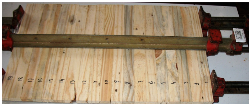
Figure 2. Pressing procedure of the core battens.
