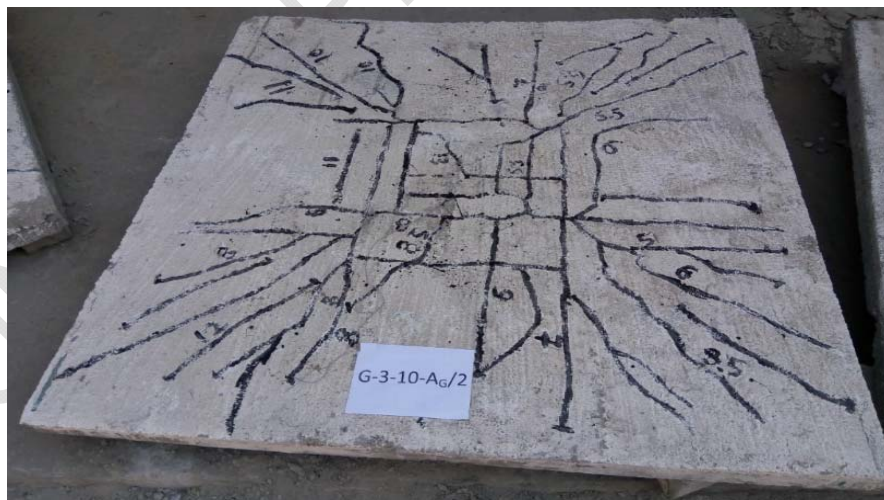
352 353 354 355 356 357 358 Fig. 19. Cracking pattern of specimen (G-3-10-Ag/2).
