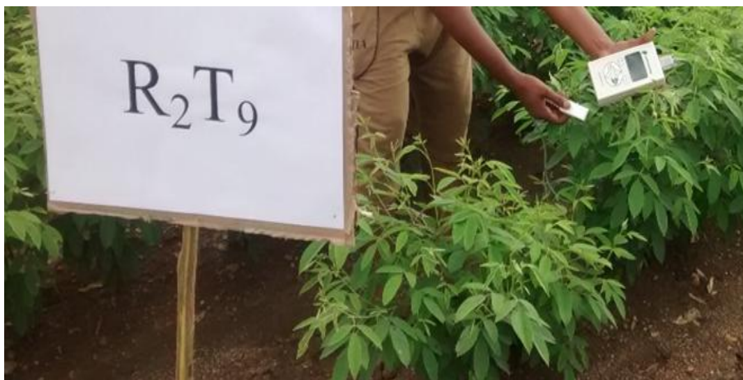
Fig. 2. Leaf Porometer (SC-1 porometer, Decagon Devices, Pullman, WA, USA) used during the experiment
