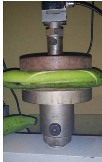
Fig. 1. Plantain hand undergoing quasi compression testing
