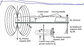
Fig. 2. Schematic diagram of the EM-38, which is 1 m in length. Tx is the transmitting coil and Rx is the receiving coil. Locations CP and Rx are where the temperature sensors were placed.
