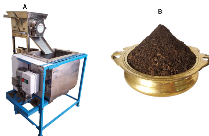
Fig.1. Waste processing machine (modified model) used for the rapid processing of degradable solid waste to organic fertilizer (A), rapid organic fertilizer produced by thermochemical conversion (B)
