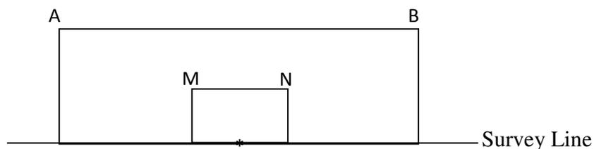
127 **Fig. 3: Schematic diagram of the Schlumberger electrode configuration used in the study.**
