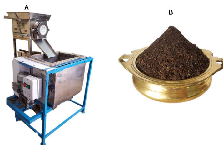
37 38 39 Fig.1. Waste processing machine (modified model) used for the rapid processing of 40 degradable solid waste to organic fertilizer (A), rapid organic fertilizer produced by 41 thermochemical conversion (B) 42
