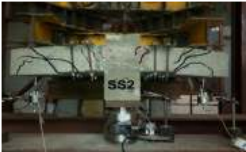
620 621 Fig. 28. Cracking pattern of specimen (SS2). 622
