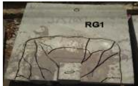
633 634 Fig. 29. Cracking pattern of specimen (RG1). 635
