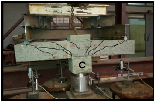
Fig. 22. Cracking pattern of specimen (C).
