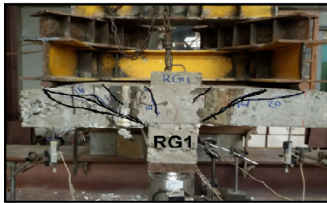
633 634 Fig. 29. Cracking pattern of specimen (RG1). 635
