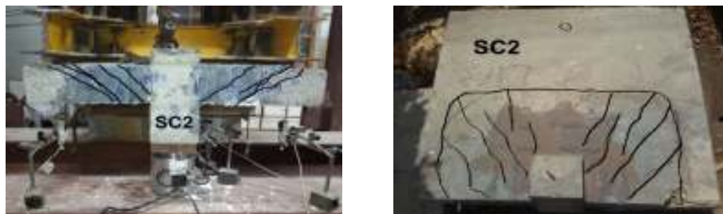
Fig. 27. Cracking pattern of specimen (SC2).
