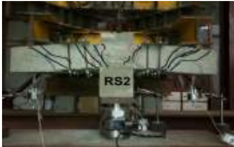
Fig. 34. Cracking pattern of specimen (RS2).
