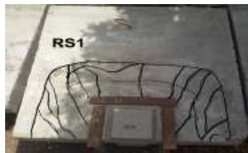
658 659 Fig. 31. Cracking pattern of specimen (RS1). 660 661
