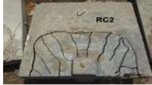
Fig. 33. Cracking pattern of specimen (RC2).
