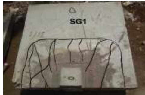
Fig. 23. Cracking pattern of specimen (SG1).
