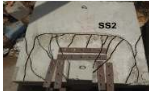
620 621 Fig. 28. Cracking pattern of specimen (SS2). 622
