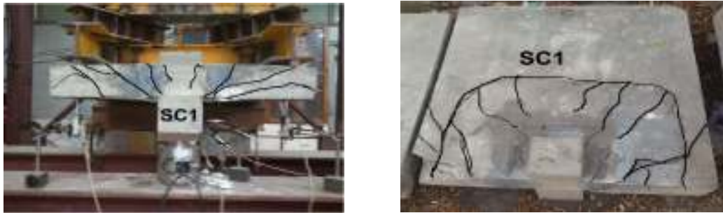
Fig. 24. Cracking pattern of specimen (SC1).
