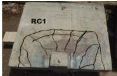
647 Fig. 30. Cracking pattern of specimen (RC1). 648
