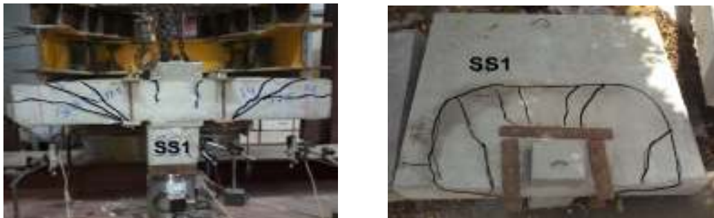
Fig. 25. Cracking pattern of specimen (SS1).
