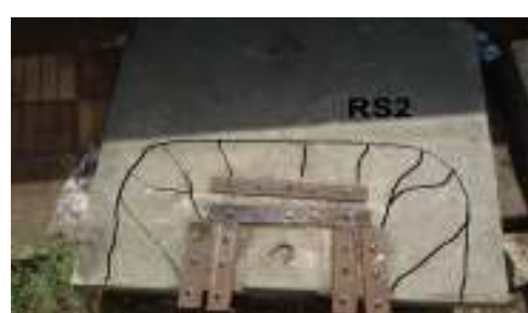
Fig. 34. Cracking pattern of specimen (RS2).
