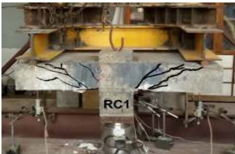
647 Fig. 30. Cracking pattern of specimen (RC1). 648
