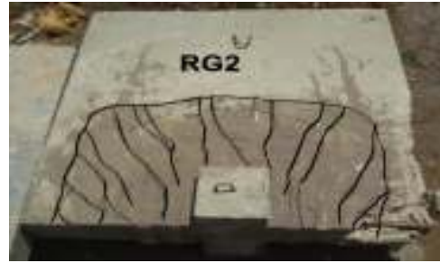
Fig. 32. Cracking pattern of specimen (RG2).
