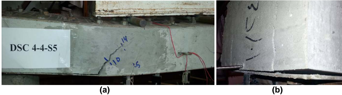
Fig. 11. View after failure load of the specimen DSC 4-4-S5 with wide crack in concrete (a), and close up view of the right side corner showing longitudinal cracks in concrete (b).
