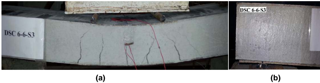
Fig. 14. View after failure load of the specimen DSC 6-6-S3 with wide crack in concrete (a), and close up view of the right corner showing slide between concrete and steel plate (b).
