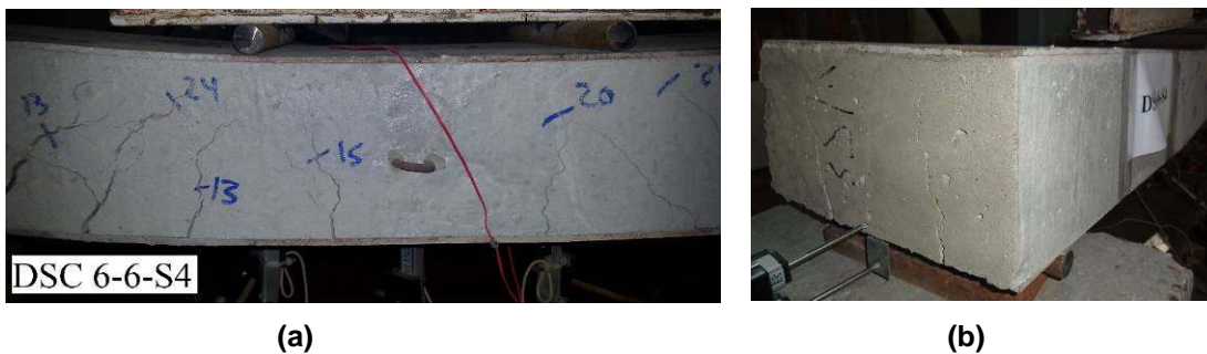
Fig. 15. View after failure load of the specimen DSC 6-6-S4 with wide crack in concrete (a), and close up view of the right side corner showing longitudinal cracks in concrete (b).
