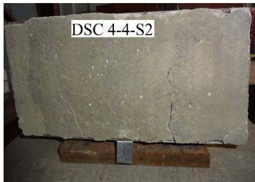
(b) Splitting cracks in concrete core.
