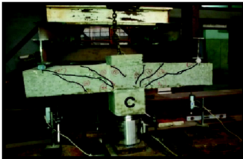
Fig. 20. Cracking pattern of specimen (C).
