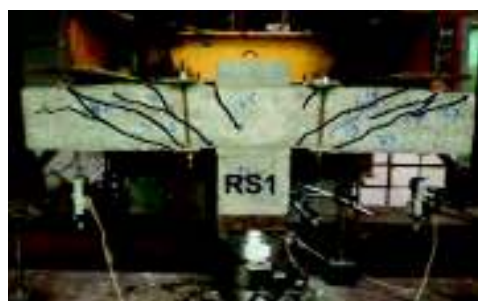
Fig. 29. Cracking pattern of specimen (RS1).
