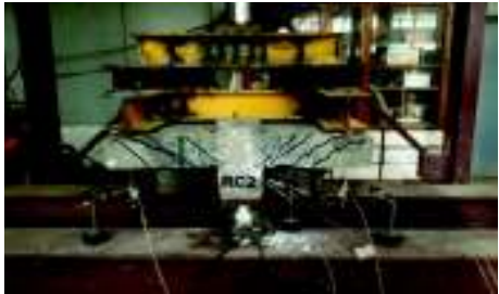
Fig. 31. Cracking pattern of specimen (RC2).
