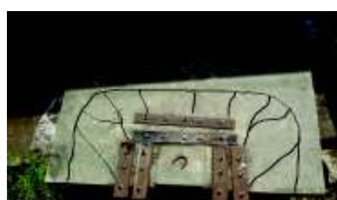
Fig. 32. Cracking pattern of specimen (RS2).
