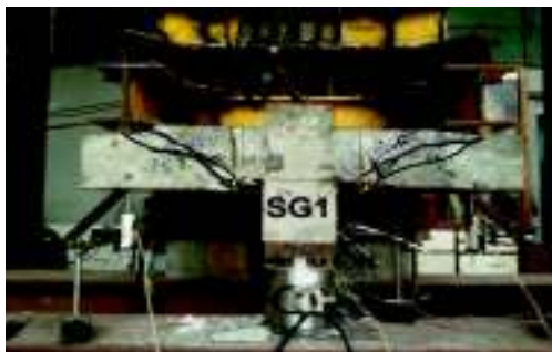
Fig. 21. Cracking pattern of specimen (SG1).
