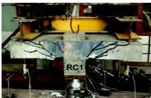
Fig. 28. Cracking pattern of specimen (RC1).
