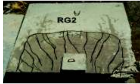
Fig. 30. Cracking pattern of specimen (RG2).
