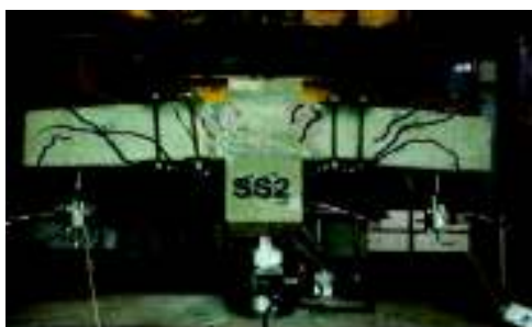
Fig. 26. Cracking pattern of specimen (SS2).
