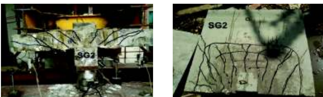
Fig. 24. Cracking pattern of specimen (SG2).
