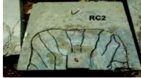
Fig. 31. Cracking pattern of specimen (RC2).
