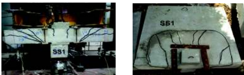
Fig. 23. Cracking pattern of specimen (SS1).
