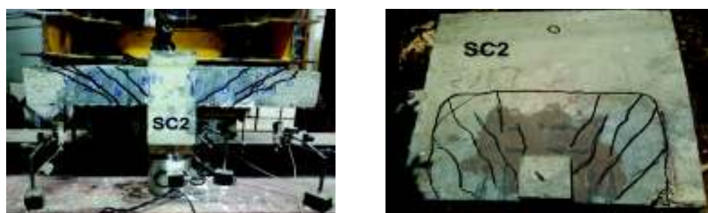
Fig. 25. Cracking pattern of specimen (SC2).
