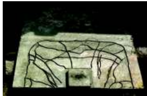
Fig. 20. Cracking pattern of specimen (C).
