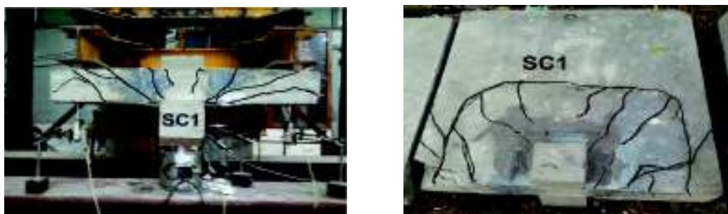
Fig. 22. Cracking pattern of specimen (SC1).
