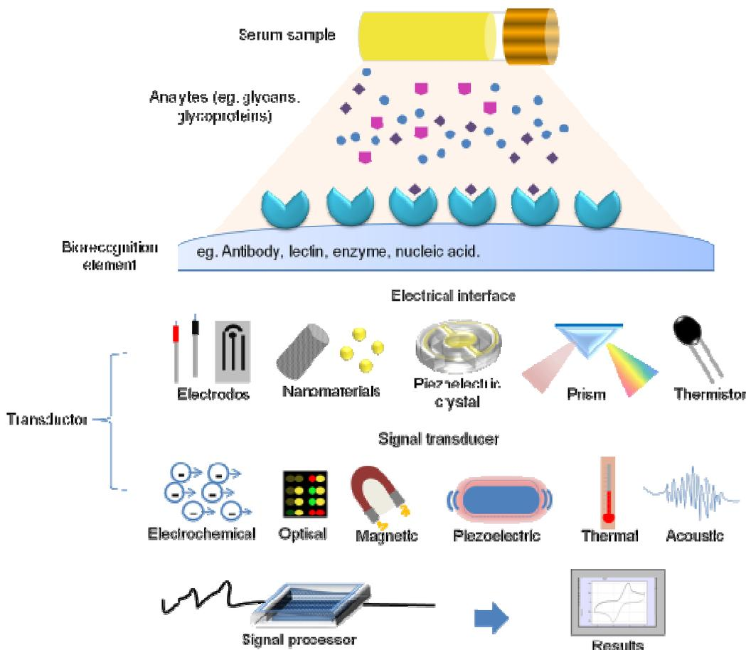
**Figure 4. Scheme of a biosensor with a biorecognition element immobilized on the solid surface in direct contact with an electrical interface of the transducer and a signal processor.**
