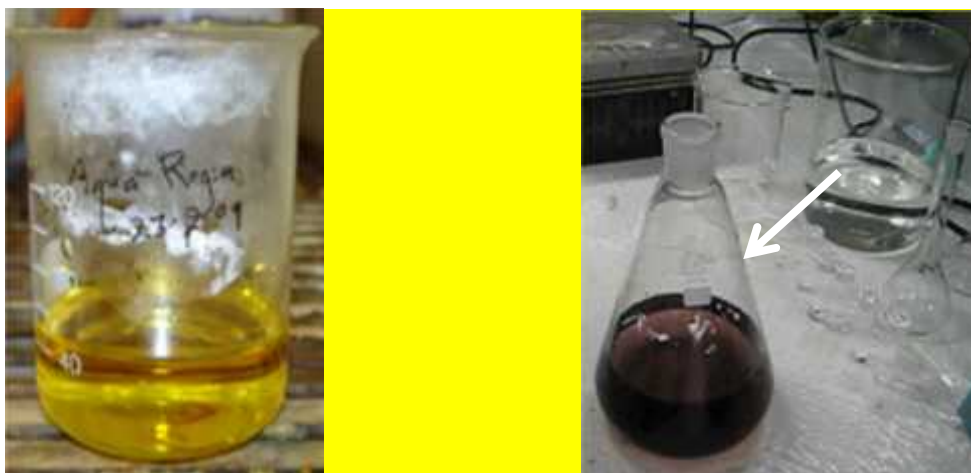
(a) Aqua Regia solution with dissolved gold precipitate (b) Colour transition during gold nanoparticles formation
