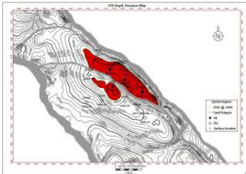
217 Figure 5: D10 Depth structure map with the wells tops and hydrocarbon contacts
